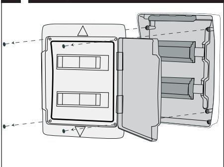
Fix the cover by the mean of 4 screws (supplied).
