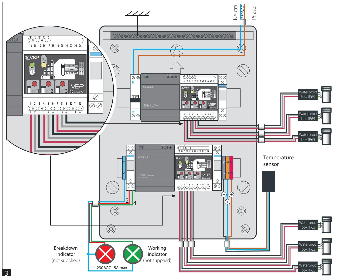
Connect the external components to the electrical box as indicated on the diagram of connection:
